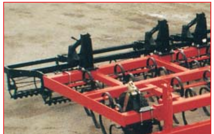
Double rouleaux crantés arrières (option) Rear notched double roll (in option) Hintere gezackte doppeltewalze
